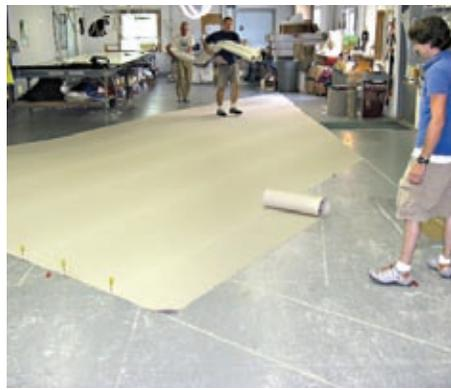
On the sail loft floor, a sailmaker lays out and cuts individual panels of sailcloth to a full-size template of the mizzen sail. These individual pieces of sailcloth are machine-sewn together to form the "membrane" of the sail.
