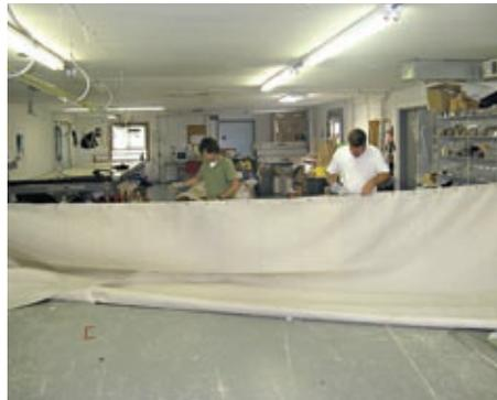
Sailmakers prepare for hand-sewing bolt rope around the perimeter of the spritsail. Bolt rope reinforces the edge of the sail and transfers wind energy to the rigging to drive the ship through the water.
