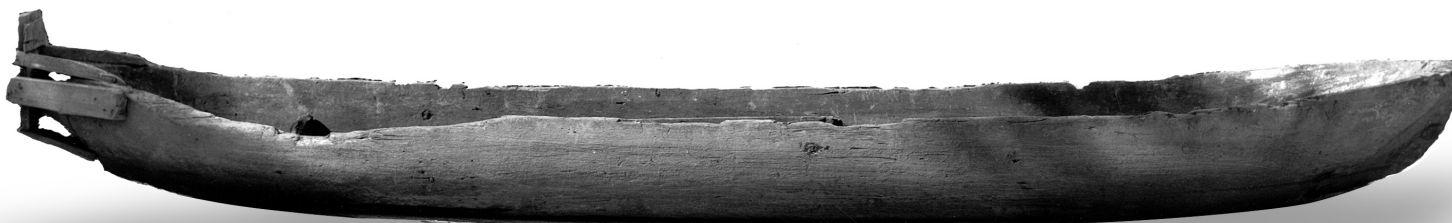
This cypress dugout canoe, measuring 17½ feet in length, was built in the late 19th century and used to navigate the shallow waterways of the Dismal Swamp. This view of the canoe shows how it was adapted over time to fit an outboard motor.
